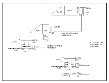
Figure 33 - ORION Dual Control Unit Front Mount/Remote Mount Installation Configuration
